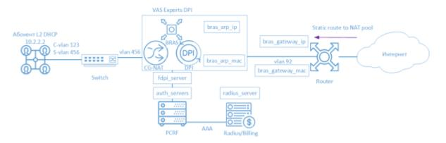
BRAS ARP L2 means that the subscriber configures the static IP address on his device. When a subscriber sends an ARP request to his default gateway, he gets to AAA in Billing. Then the subscriber is terminated by Stingray Service Gateway (SSG) and transferred to border equipment. A scheme when subscribers are given the /30 prefix is also possible.
