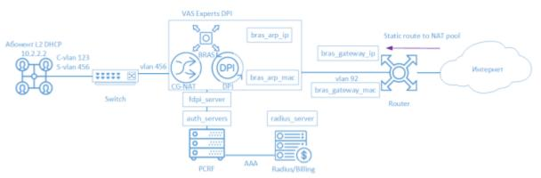
FastDPI BNG/BRAS supports PPPoE connection since version 7.2. The subscriber connects to the Stingray Service Gateway (SSG) using the PPPoE connection type, is terminated by SSG and then gets to the border. The following elements are involved in the SSG operation scheme in BNG/BRAS PPPoE mod:
