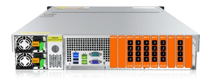
Cards with 10/25/40/100 network ports are placed in **slots 1-10**Each slot has a unique PCle bus identifier, e.g. **02:00**.
