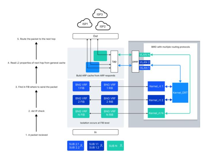
The prefix Lite means that SSG only separates routing tables, but does not place the traffic of an individual VRF into a unique tunnel (MPLS, VXLAN). VRF Lite allows isolating the services provided between each other and optimizing routing when using different links.
