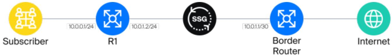
On R1, our border is the gateway. In order to ensure the passage of traffic from the Internet to subscribers, it is necessary to add a route on the border: ip route add 100.0.0.0/24 via 10.0.1.2 After that, the traffic for the NAT pool will be routed from BR to R1, on the way to which it will be NATed when it gets to DPI. Traffic to addresses without NAT translation will be dropped on SSG.
