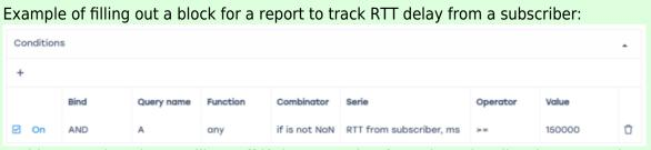
In this case, the trigger will go off if the RTT value from the subscriber is greater than or equal to 150000 ms in the table from step 2.
